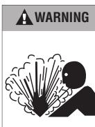
Hazardous pressure. Do not run pump against closed discharge. Release all system pressure before working on any component.
